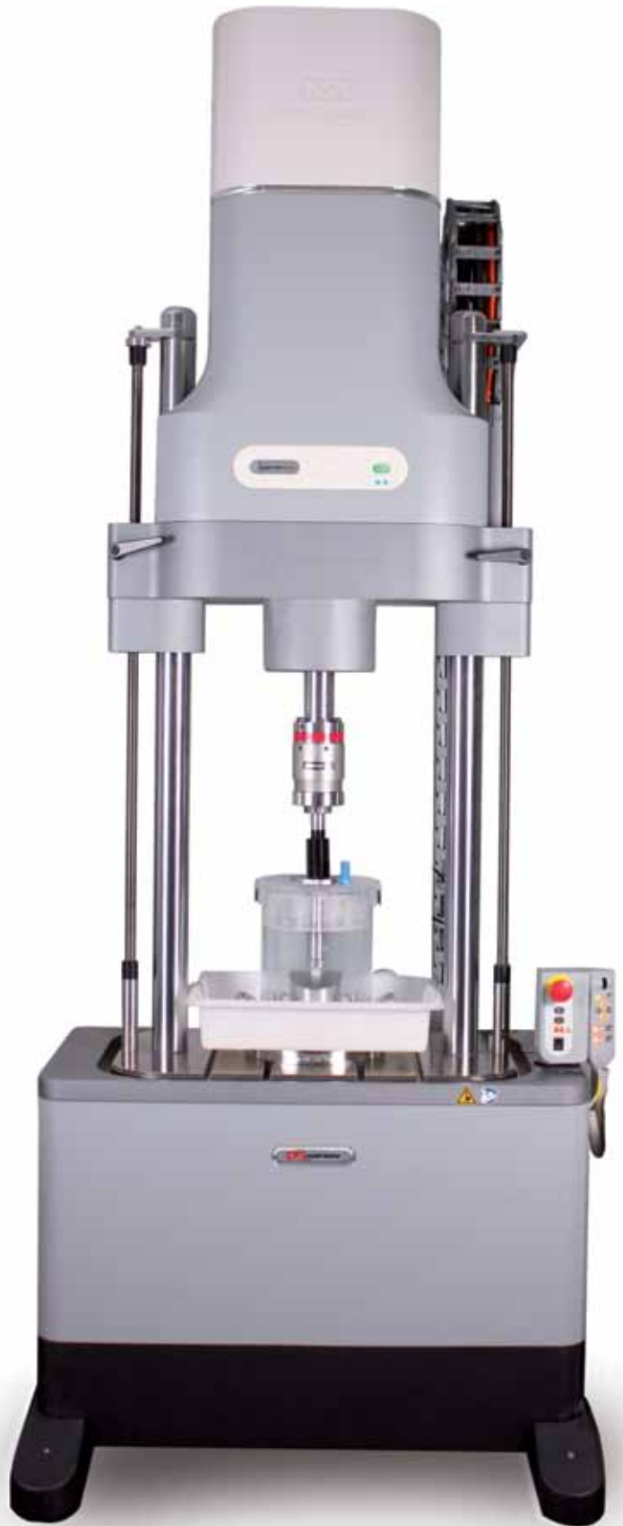
Dental implants are tested to ISO 14801 within a saline bath on ElectroPuls dynamic instruments to evaluate effects of corrosion fatigue
