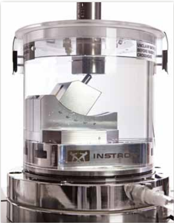
Pre-angled dental implants can be tested using a variable angle fixture within a fluid bath to ISO 14801
