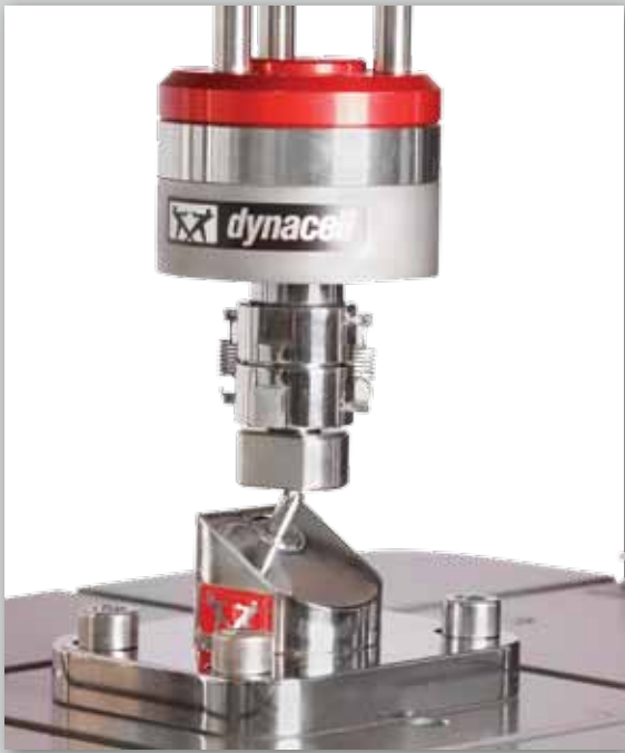
A 30 ° fixed angle fixture is used for testing of straight endosseous dental implants to ISO 14801
