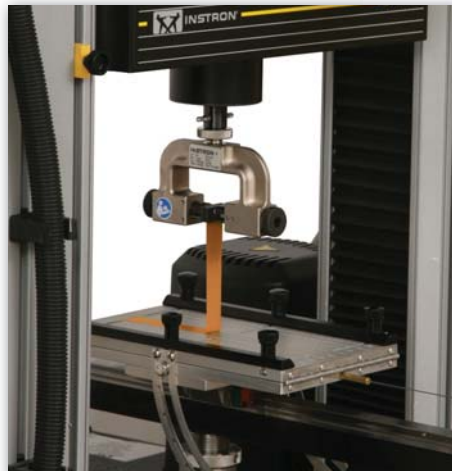
90° peel adhesion test according to ISO 813
