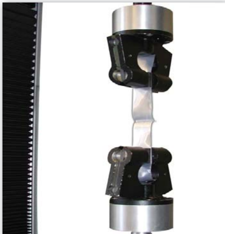
180° peel adhesion test according to ASTM D1876
