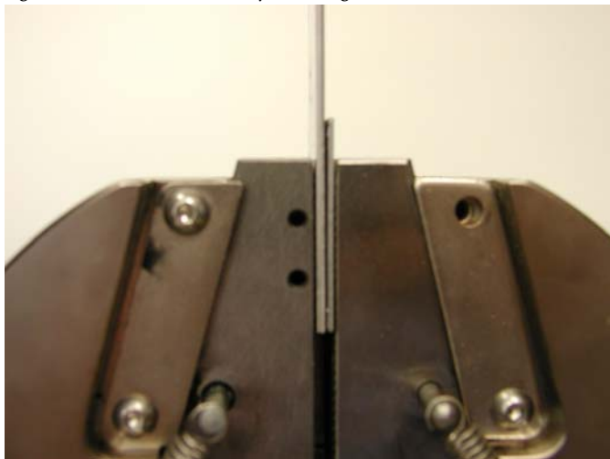
▲ Figure 1: Close-up of test configuration. Note the spacer within the grip faces used to properly align the specimen.
