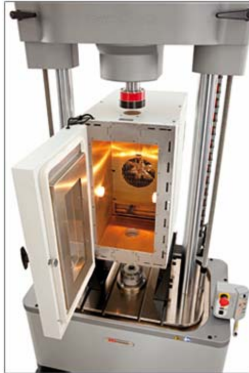
3119-505 Environmental Chamber fitted on an ElectroPuls E10000
