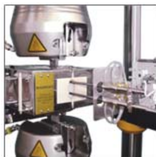
Furnace with External Grips and Extensometer
