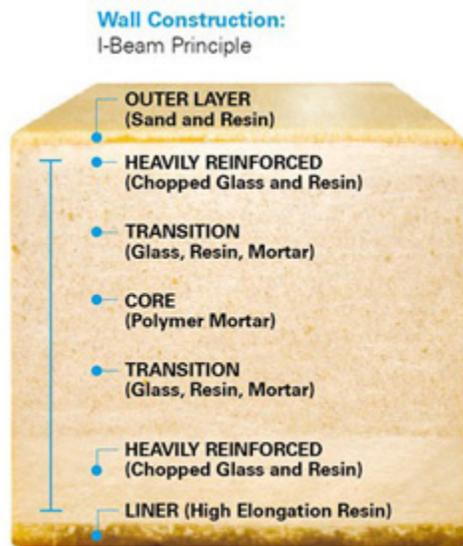
Illustration of a typical HOBAS pipe wall composition
