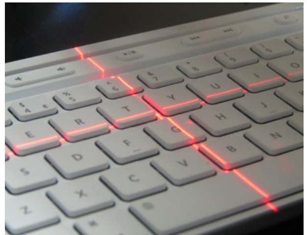
Laser crosshair that gives a precise indication of the contact point
