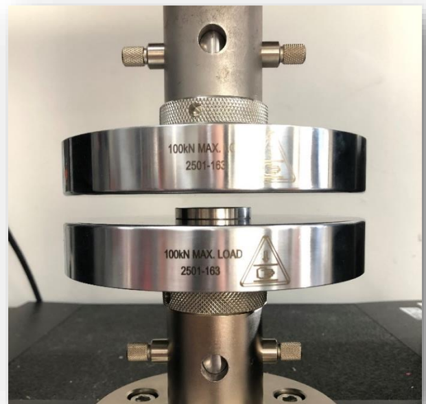
Figure 3 – Dummy Specimen - Hardened Steel Disc, Compression Test
