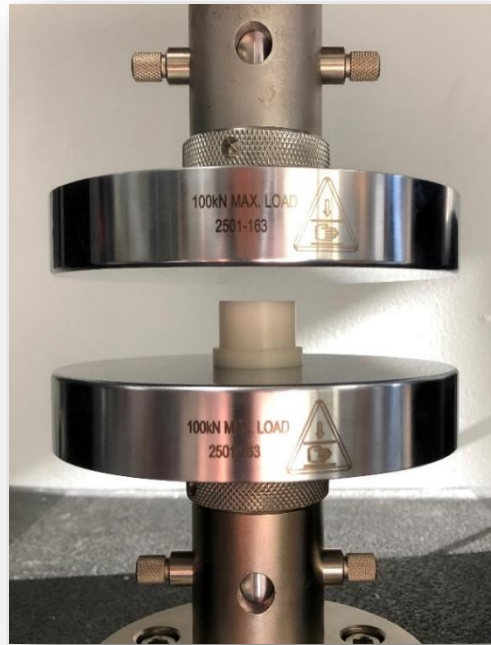
Figure 5 - Plastic component, ready for test
